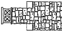
C FALSE CHIMNEY CAP WITH METAL GRILLE STONE VENEER @ CHIMNEY BASE (COBBLESTONE BY ELDORADO STONE)
