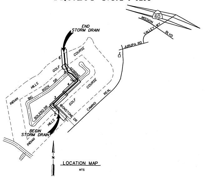
Pedley Hills Bolero Drive Storm Drain, Stage 1 is located in the Pedley Hills area of Riverside County and consists of constructing approximately 1,560 lineal feet of mainline storm drain ranging from 24—inch to 36—inch diameter. Also included in this project are several inlets and an outlet structure located southerly of Ironstone Drive.
