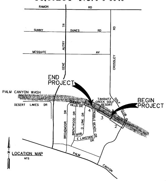
Palm Canyon Wash/Levee Restoration, Stage 91 consists of constructing approximately 1200 feet of earthen fill to raise the existing earthen/grass lined levee a maximum of 2.5 feet. Transverse concrete golf cart paths will be rebuilt to match new grade.
