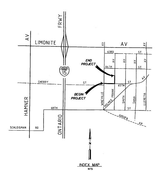
DAY CREEK - FRANK AVENUE STORM DRAIN IS LOCATED WITHIN THE UNINCORPORATED MIRA LOMA COMMUNITY OF RIVERSIDE COUNTY AND CONSISTS OF APPROXIMATLEY 1,100 LINEAL FEET OF 18-INCH DIAMETER REINFORCED CONCRETE PIPE. THIS PROJECT IS AN UNDERGROUND SYSTEM DESIGNED TO DRAIN THE EXISTING SUMP AREA LOCATED ON THE WEST SIDE OF FRANK AVENUE BETWEEN 64TH AND 65TH STREETS.
