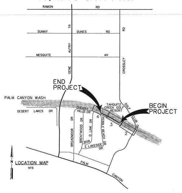
Palm Canyon Wash/Levee Restoration, Stage 91 consists of constructing approximately 1200 feet of earthen fill to raise the existing earthen/grass lined levee a maximum of 2.5 feet. Transverse concrete golf cart paths will be rebuilt to match new grade.
