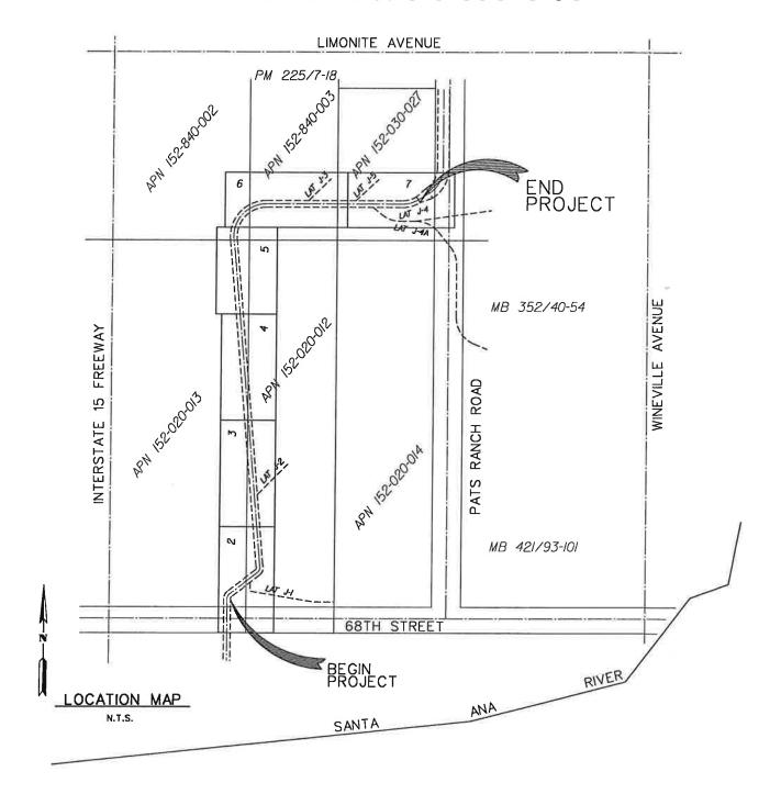
Day Creek MDP Line J, Stage 2 consists of constructing approximately 1,900 lineal feet of 12'H x 6'W reinforced concrete box in the city of Jurupa Valley. The alignment for the project begins at the Caltrans culvert under 68th Street and proceeds north for approximately 1,300 lineal feet as it parallels the east side of the I-15 freeway, then turns east for approximately 600 lineal feet where it ties into the existing Stage 1 portion of project in Pats Ranch Road.
