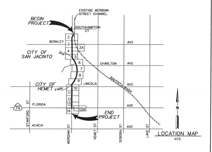
The Proposed Project is located in Zone 4, primarily within the City of Hemet, with small portions extending into the City of San Jacinto and into Unincorporated County of Riverside. This project will construct approximately one mile of underground storm drain extending from Meridian Street Channel south of South Hampton Court and then southerly along Meridian Street and Park Avenue. The storm drain will terminate approximately 200 feet south of Florida Avenue.
