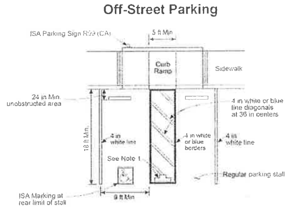
Figure 3B-22 (CA). Examples of Disabled Persons Parking Symbol, Legend and Related Markings (Sheet 2 of 2)
