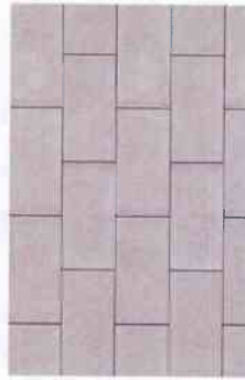
3 8" SMOOTH FACE C.M.U., STUCCO FINISH, PAINT PER EXTERIOR EXTERIOR ELEVATIONS EXHIBIT B
