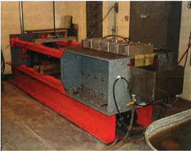
Fig 7. Large-diameter cyclic direct shear machine used by Nye and Fox (2007).
