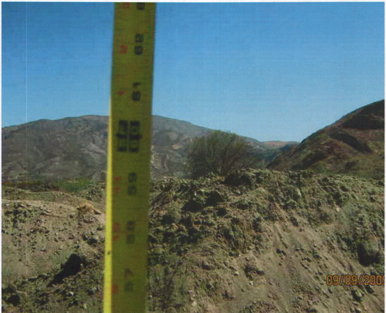
STOCK PILES MEASURED APPX. 5' HIGH PILES - 09/09/2009
