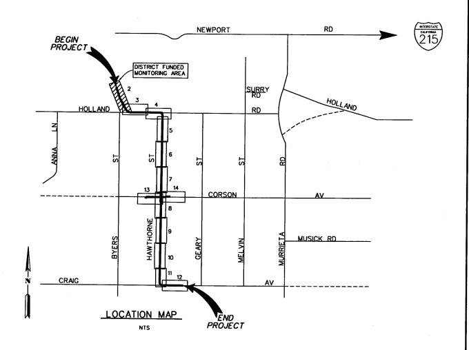
Menifee—Hawthorne Avenue Storm Drain, Stage 1 is located within the city of Menifee and consists of constructing approximately 3,900 lineal feet of mainline storm drain ranging from 48—inch to 78—inch diameter. Also included in this project are several inlets and an outlet structure located northerly of Holland Road.
