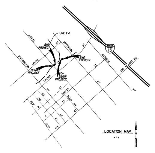
Murrieta Line F Channel Repair is located within the city of Murrieta and consists of repairing approximately 150 lineal feet of trapezoidal concrete lined channel and approximately 200 lineal feet of trapezoidal concrete channel slope paving and gabion invert construction.
