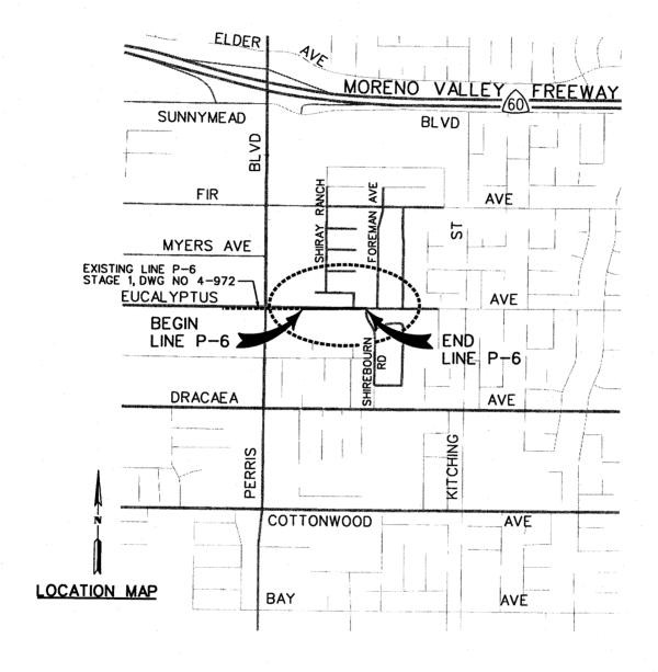
Sunnymead MDP Line P-6, Stage 2 — This project is an underground storm drain approximately 700 lineal feet of reinforced concrete pipe ranging in size from 36" to 24". The project starts approximately 600 lineal feet east of the intersection of Perris Boulevard and Eucalyptus Avenue and ends at the intersection of Eucalyptus Avenue and Shirebourn Road in the city of Moreno Valley. It will tie into the existing storm drain facility of Sunnymead MDP Line P-6, Stage 1.
