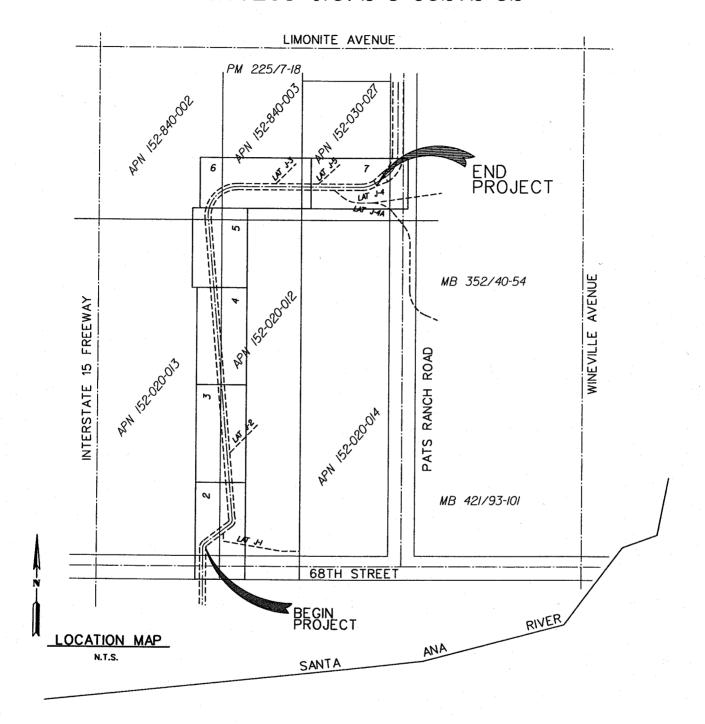
Day Creek MDP Line J, Stage 2 consists of constructing approximately 1,900 lineal feet of 12'H x 6'W reinforced concrete box in the city of Jurupa Valley. The alignment for the project begins at the Caltrans culvert under 68th Street and proceeds north for approximately 1,300 ineal feet as it parallels the east side of the I-15 freeway, then turns east for approximately 600 lineal feet where it ties into the existing Stage 1 portion of project in Pats Ranch Road.
