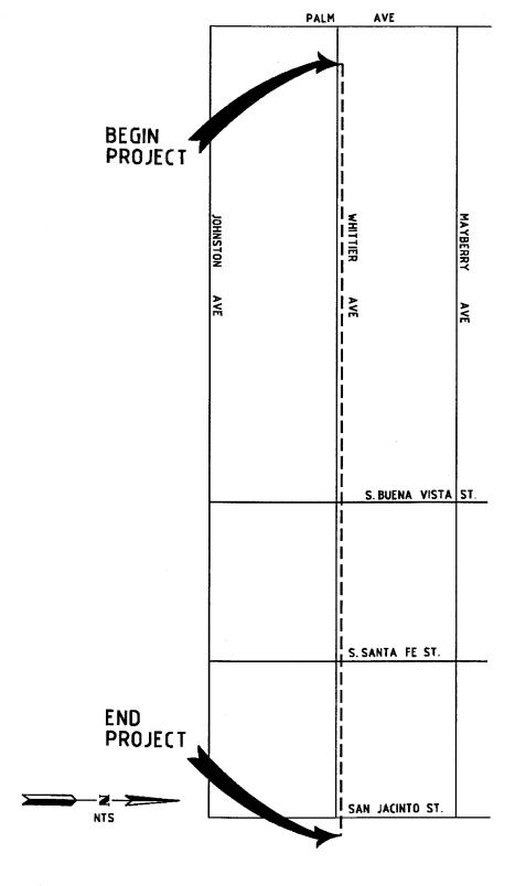
The project consists of the construction of approximately 6,600 linear feet of reinforced concrete pipe ranging from 18 inch to 78 inch in diameter. The project is located along Whittier Avenue between Palm Avenue and San Jacinto Street within the City of Hemet and unincorporated Riverside County near Hemet, California.
