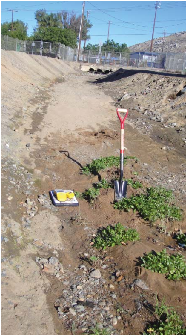
Sample Point 3. This sample point is located in the channel, just downstream from Temescal Avenue. All three wetland parameters, vegetation, soil, and hydrology, were present. The vegetation at this location was dominated by non-native wetland species. 23 December 2014
