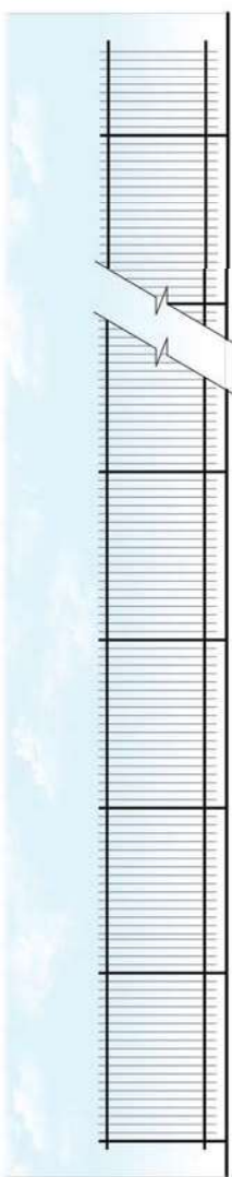
3 OPEN VIEW FENCE | 6' TUBULAR STEEL FENCE MAINTAINED AS NOTED ON PLAN N.T.S.
