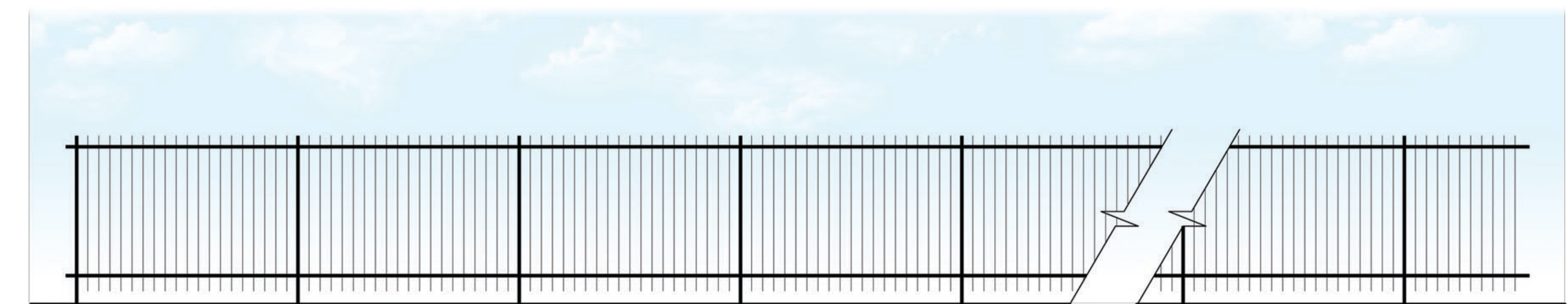
3 OPEN VIEW FENCE | 6' TUBULAR STEEL FENCE N.T.S. MAINTAINED AS NOTED ON PLAN
