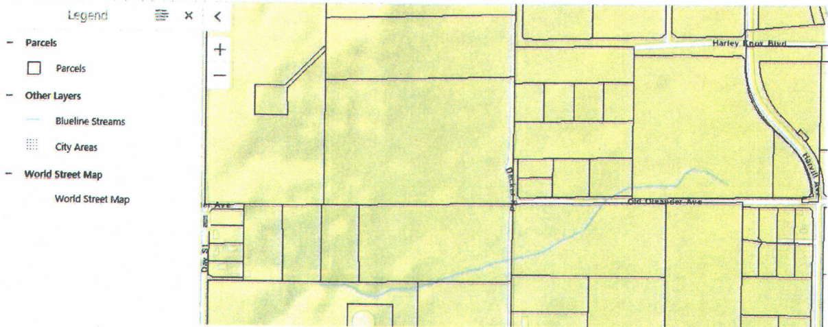
Riverside County GIS Flood Mapping clearly shows the blue line stream starting in the arroyo east of Day street and continuing across parcels that include Building "E" and "D".
