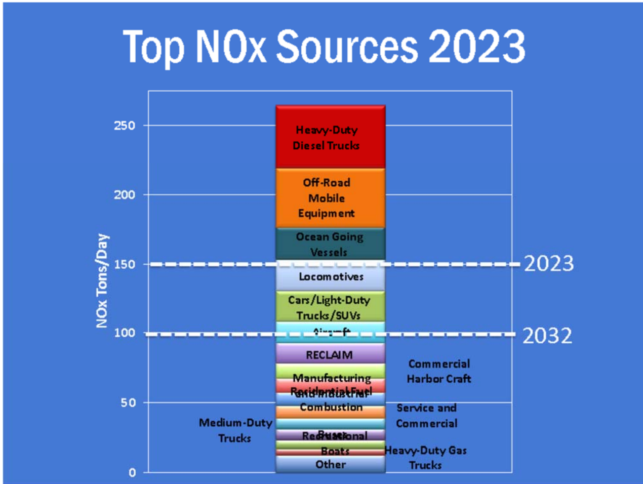
Figure 1. Top Sources of NOx, in the South Coast Air Basin and Reductions Required for 2023 and 2032 to Meet Ozone Standards (Source: SCAQMD)
