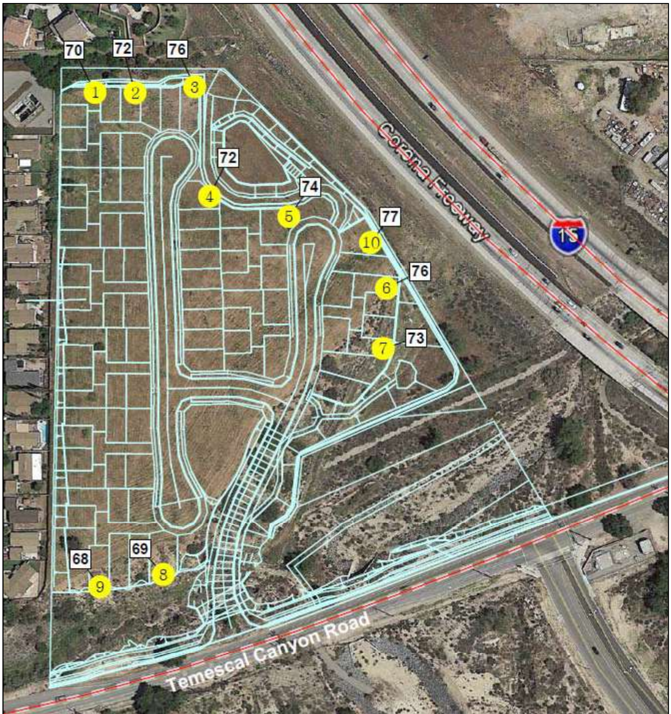
Figure 32-1 Unmitigated Traffic Noise Levels (CNEL)
