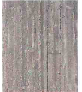
1.02 RANDOM STONE CONCRETE HORIZONTAL
