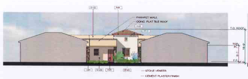
INTERIOR COURTYARD ELEVATION (WEST END)
