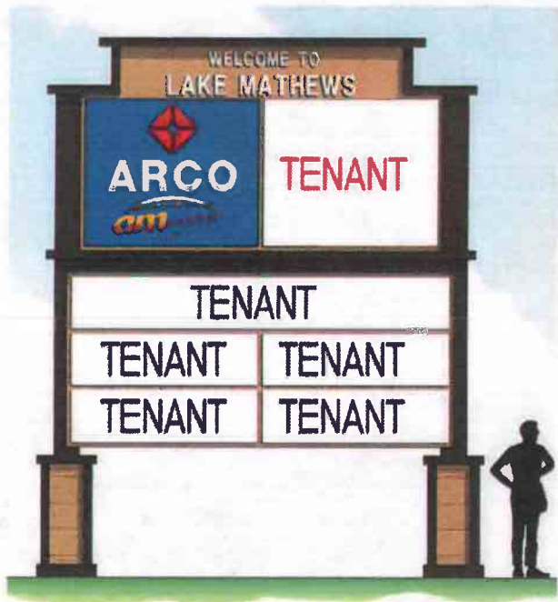
M SIGN-M: PYLON SIGN COLOR DETAIL 1/8" = 1'-0"
