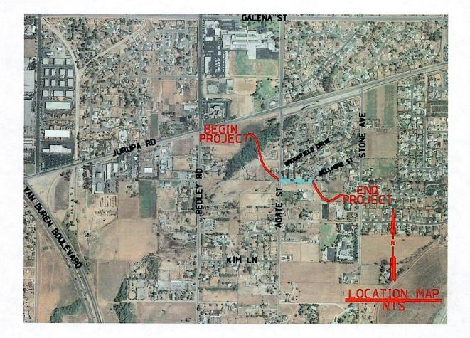
THE JURUPA-PYRITE MDP LINE A-2 PROJECT IS LOCATED IN THE CITY OF JURUPA VALLEY AND WILL SERVE TO ALLEVIATE RECURRING FLOODING ISSUES EXPERIENCED BY ADJACENT RESIDENTS. THE PROJECT WILL CONSTRUCT A 9"H X 6'W CONCRETE TRAPEZOIDAL SWALE WITH 2H:1V SIDESLOPES THAT WILL CONVEY FLOWS WEST FROM THE TERMINUS OF BELLMORE STREET AND OUTLETS THROUGH A GRATED TRENCH DRAIN SYSTEM ACROSS AGATE STREET.
