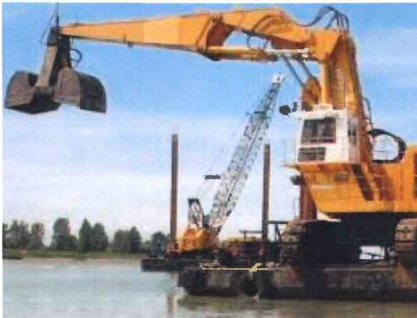
Figure 6 Typical Barge Mounted Excavator w/ Clam Shell
