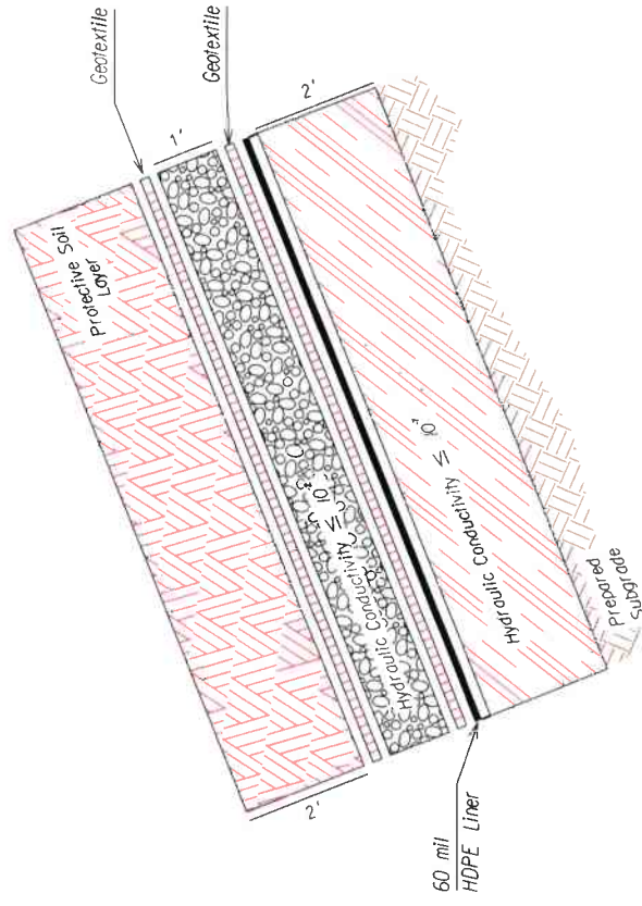
Prescriptive Side Slope Liner System
