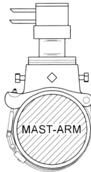
MOUNTING CLAMP FOR EVP OPTICAL DETECTOR
