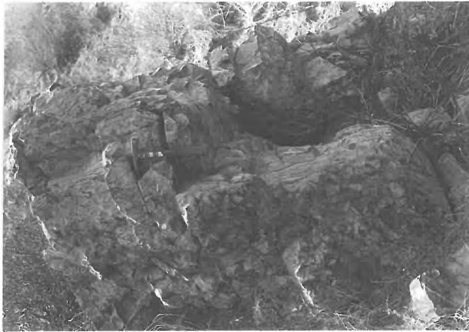
Photo 3 Photograph of metamorphic-rock outcrop at sample location HH-10a (Figure 1). Discontinuity planes at this location are not as closely spaced as at other locations, but are nevertheless unacceptably close for quarry operation. Hammer is 0.3 m (1 ft) long.
