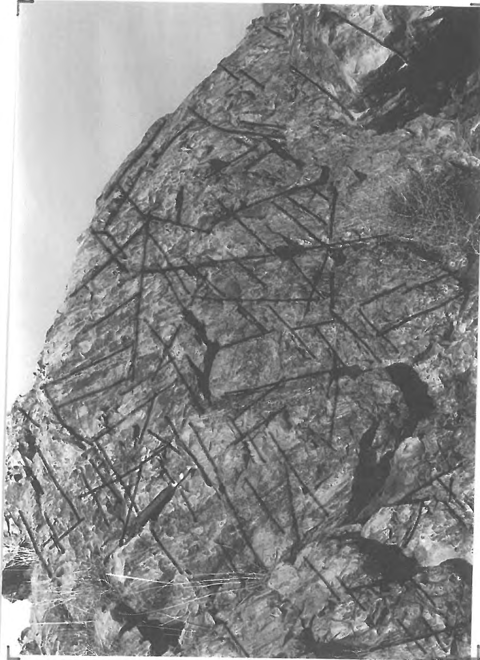
Photo 2 Photograph of metamorphic-rock outcrop at HHQS showing several discontinuity planes. Close inspection of the photograph reveals that the planes are closely spaced and at least three intersecting orientations. Hammer is about 0.3 m (1 ft) long.
