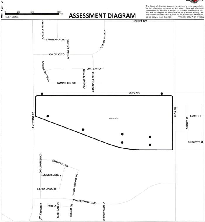
DENOTES MAINTAINED STORMWATER RUNOFF CATCH BASIN FILTER
