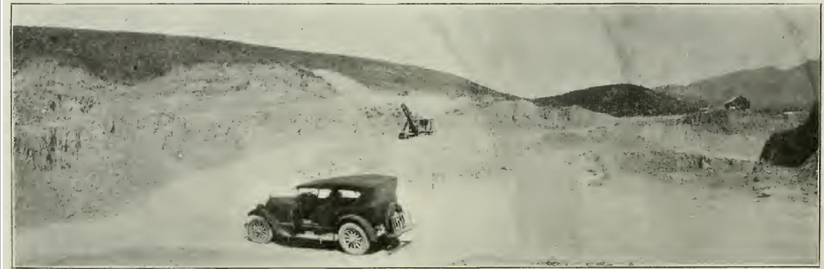
PHOTO No. 45. Emsco Clay Co. Harrington pit, facing east, 8 miles SE. from Corona, Riverside County. The shovel is standing on top of the 'Harrington No. 5' fireclay (sample No. 70) and is digging pink mottled clay (sample No. 71).
