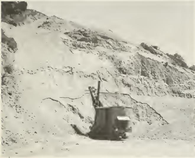
FIGURE 20. Thomas clay deposit, east pit (operated by Joe Deleo, Jr.). Fissile elaystone of the Silverado formation (Paleocene) is mined by a ripper-bulldozer which piles loosened material from hill above at foot of sloping quarry face. Loosened material is loaded by the  $1\frac{1}{2}$  cubic yard power shovel into dump trucks for transport to several manufacturers of common clay products. Observer faces southeast.
