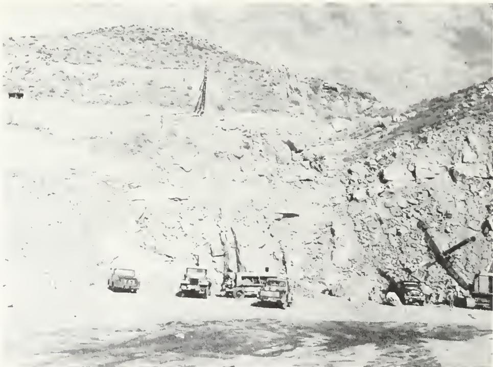
FIGURE 30. Matich and Sundt Company's Temescal Canyon quarry, south pit, September 1957. Most of the rock quarried here is granodiorite but the ravine (right center) contains a small body of quartz latite porphyry. Blast holes are drilled above (center) while blasted-down rock is loaded below (lower right) for transport to sizing area. Observer faces east.
