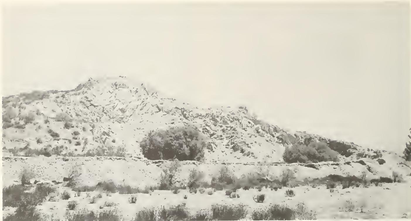
FIGURE 24. Jameson quarry, west of Home Gardens. Cretaceous micropegmatite granite has been obtained here intermittently since before the early 1920's, for use as small riprap and rubble. The most extensive operation was during 1939-40 when J. B. Stringfellow Construction Company quarried a large tonnage of riprap used to face Prado Dam. Observer faces east.
