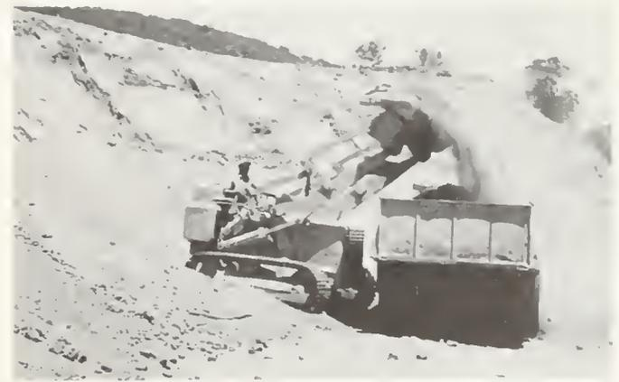
FIGURE 18. Loading clay shale, Sky Ranch Clay Company mine, west pit. Typical method of loading clay shale in the Corona area. Observer faces northeast.
