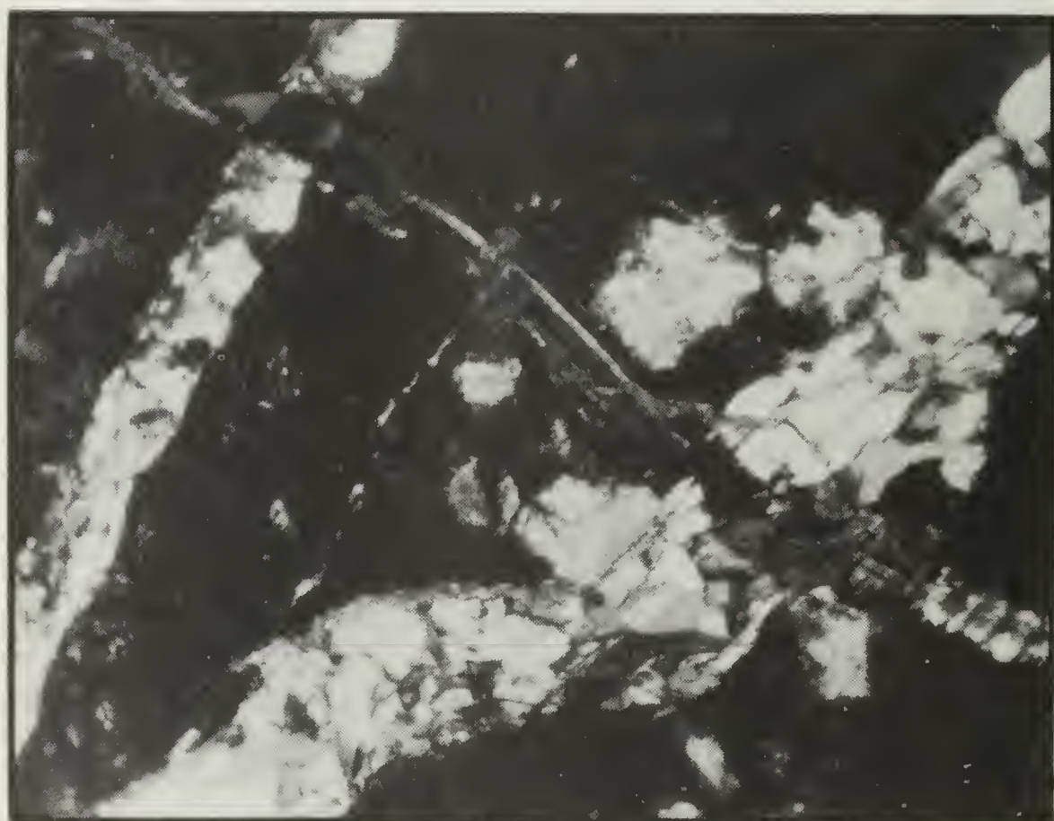
FIG. 17. Veinlets (large) of wollastonite and idocrase cutting impure partially silicated limestone or tactite (dark) and in turn cut by chalcedonic quartz veinlets. Crossed nicols. Magnification 75X.
