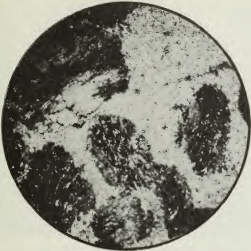
FIG. 10. Spots of wollastonite in fine-grained limestone. An early stage in the development of wollastonite tactite. Crossed nicols. Magnification 11X.
