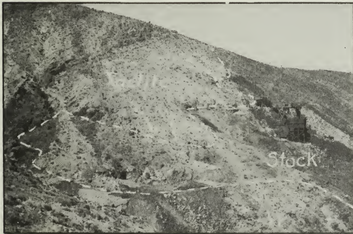
FIG. 27. View of the Independence mine (right of center) and the Essex mine (lower left). The prominent white tactite outcrop in the center of the picture lies as a blanket over the large Independence orebody within the ridge and a part of which may outcrop in the dark area in the extreme left in the picture.
