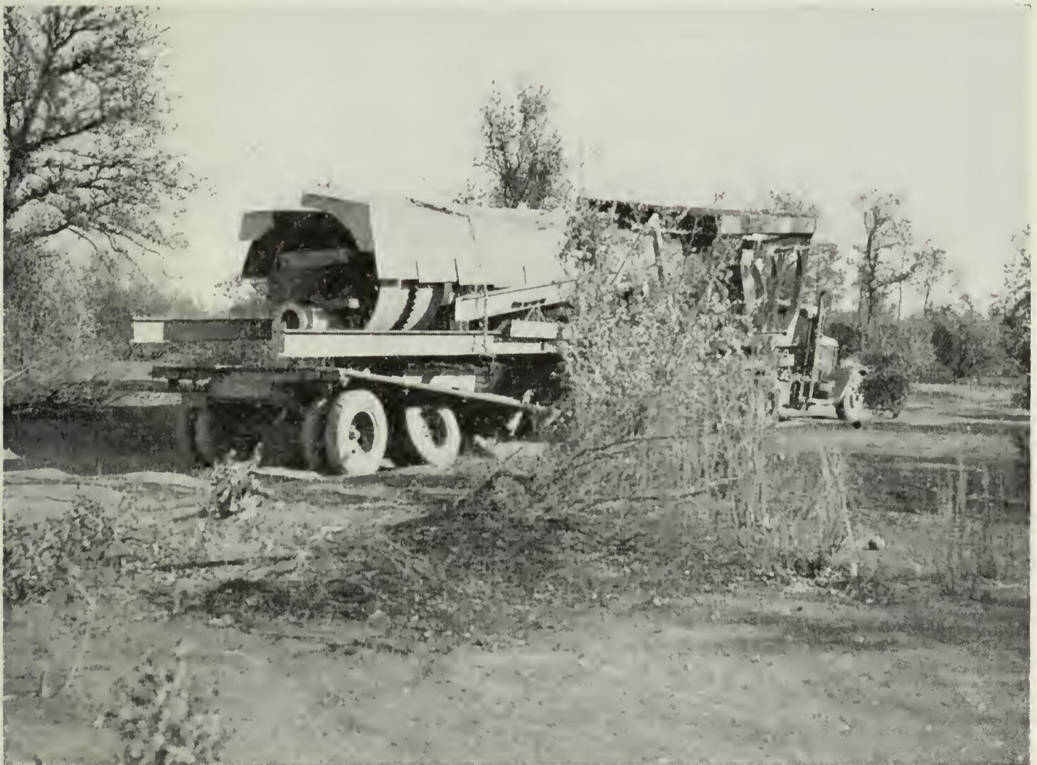
PHOTOGRAPH 4. Trommel for dragline dredge on truck and trailer.
