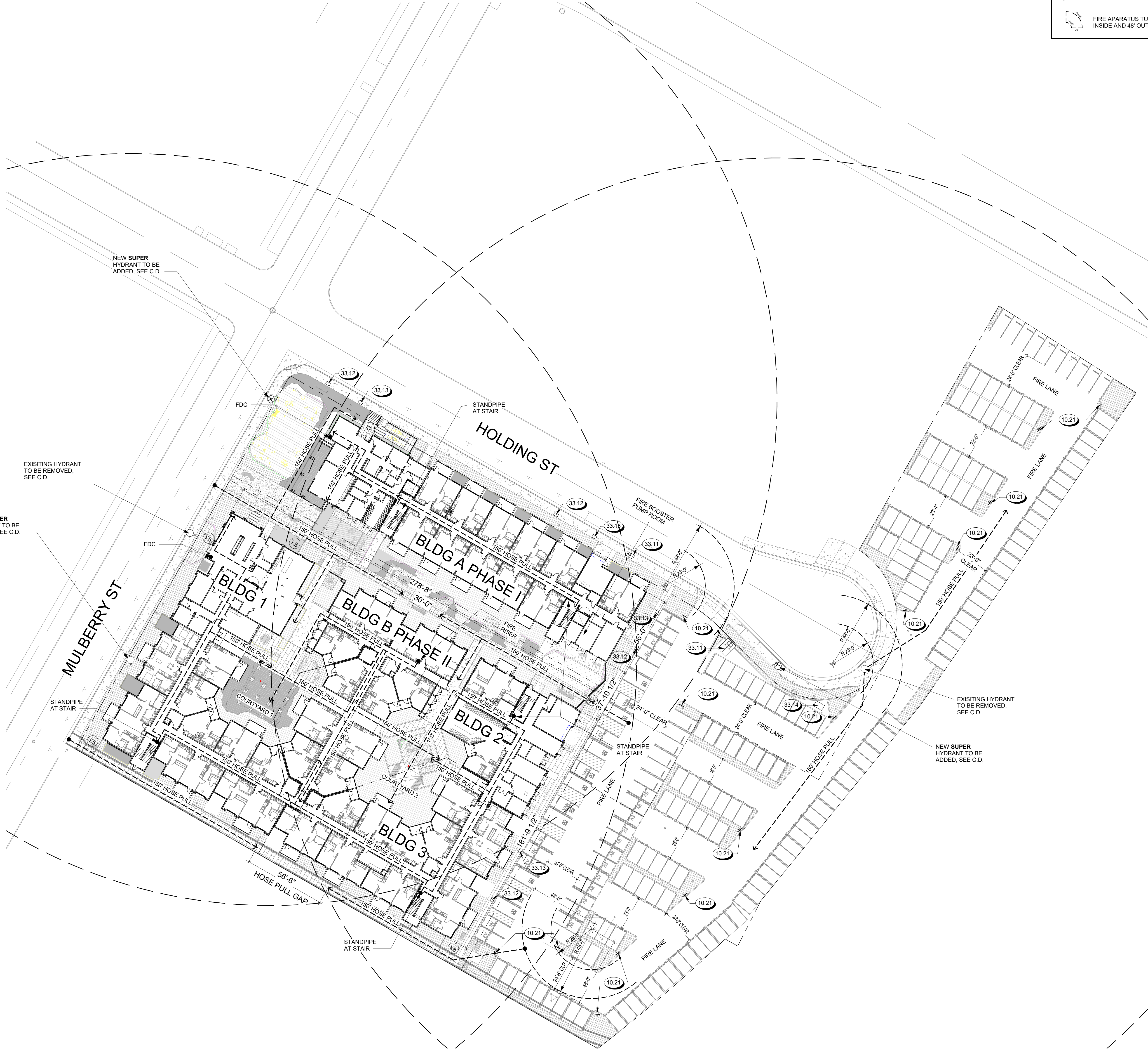
1 FIRE ACCESS SITE PLAN - PHASE I 1" = 30'-0"
