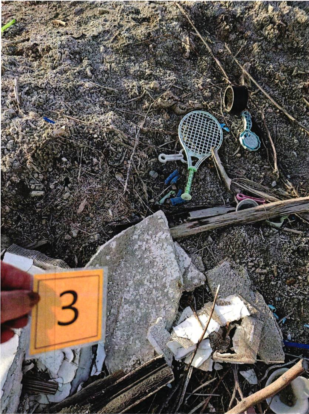
Photograph 3 – illustrates sample TB3 white, acoustical ceiling from Zone B, asbestos present (5% Chrysotile).
