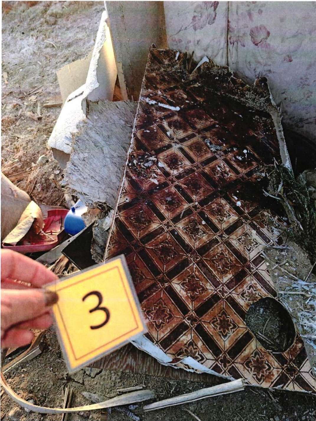
Photograph 6 – illustrates sample TG3 tan/brown, sheet vinyl from Zone G, asbestos present (10% Chrysotile).
