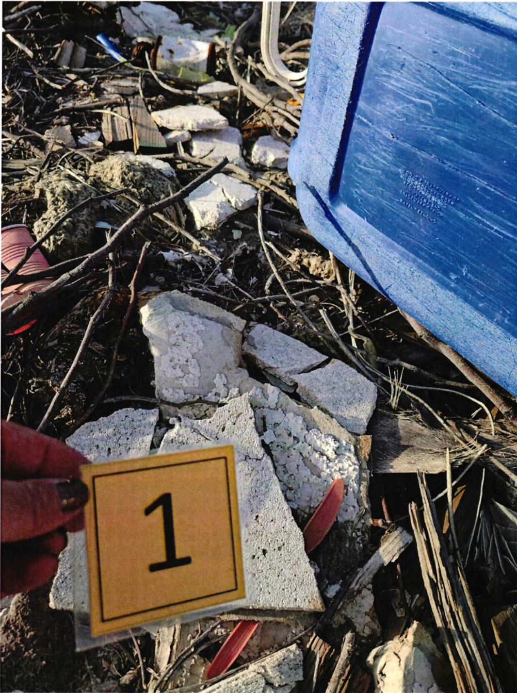
Photograph 1 – illustrates sample TB1 white, acoustical ceiling from Zone B, asbestos present (5% Chrysotile).
