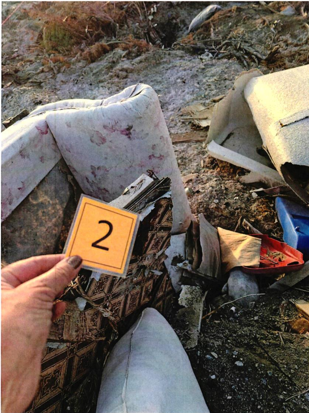
Photograph 5 – illustrates sample TG2 tan/brown, sheet vinyl from Zone G, asbestos present (10% Chrysotile).
