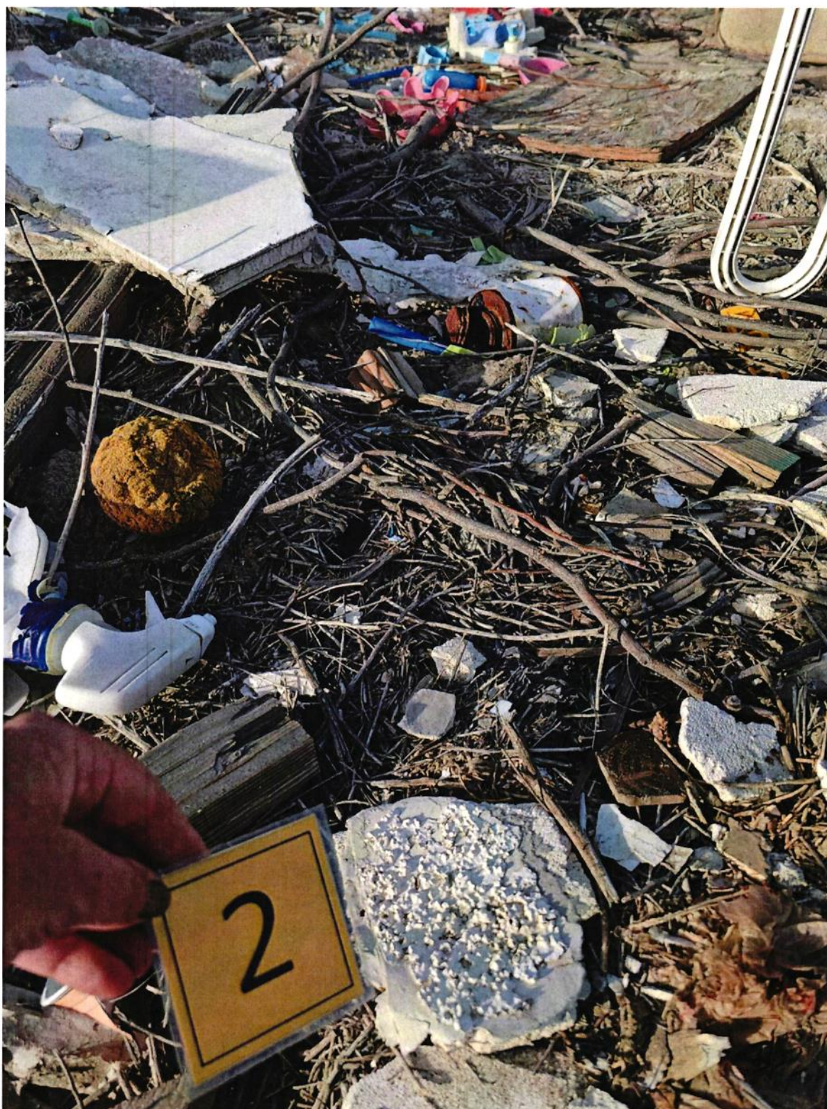
Photograph 2 – illustrates sample TB2 white, acoustical ceiling from Zone B, asbestos present (5% Chrysotile).
