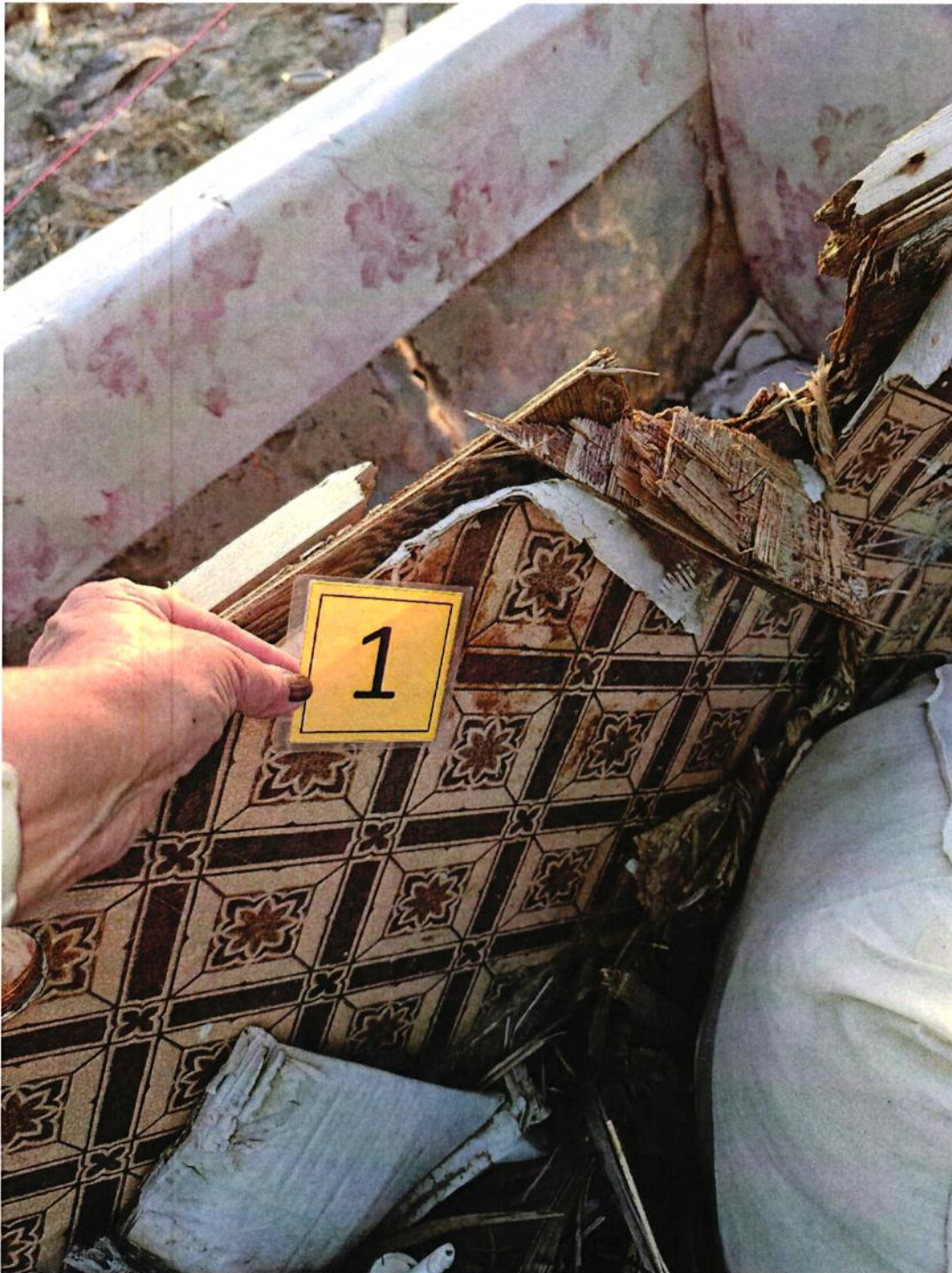
Photograph 4 – illustrates sample TG1 tan/brown, sheet vinyl from Zone G, asbestos present (10% Chrysotile).
