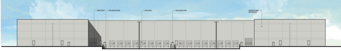
NORTH ELEVATION 36' CLEAR HEIGHT
