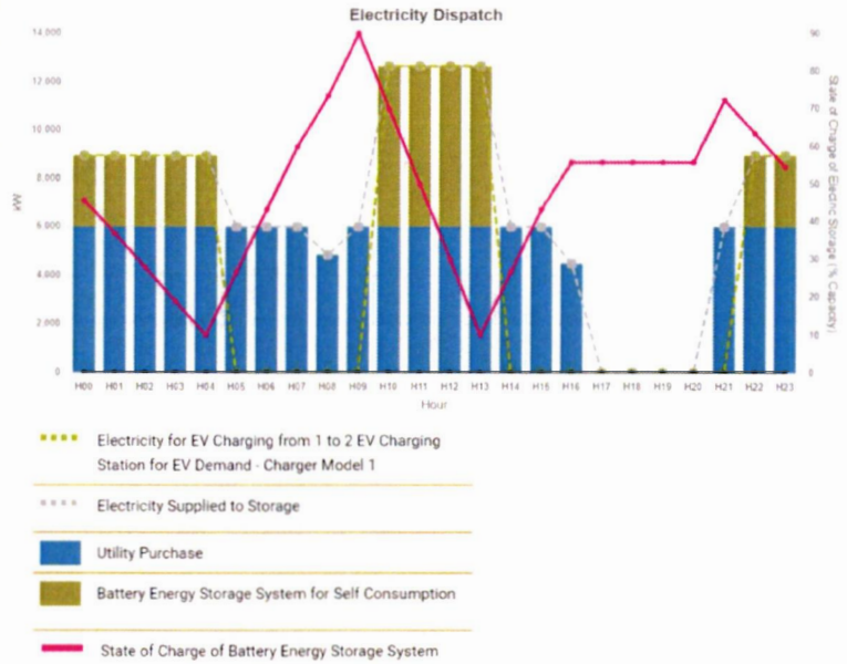
Figure 2: Example Depiction of BESS Development for EV Charging
